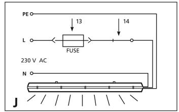
After fitting the cover, reactivate main fuse and swich. LED-Luminaries ist lightening.
