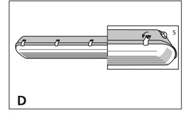
Open the cover of the lamp by using the clips.
