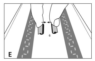
Remove the mounting plate (connected to the case through a safety cord) by pushing together the plastic hooks (6).
