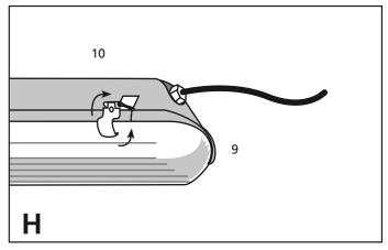
Mounting the diffusor cover on the case (10). Close the clips (11).
