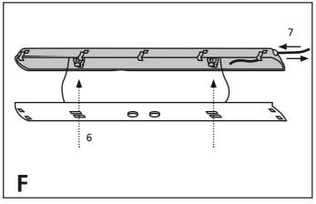
Insert the electric connecting cable through the rubber joint in the
