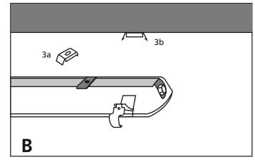
Installation of the mounting parts for wall- and ceiling. In case of hanging the lamp with a chain use extra steel eyebolts.
