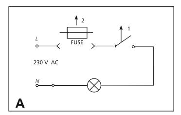
Switch off the power supply to the lamp. Disconnect the main fuse.
